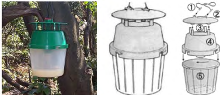
Figure 4-4. Bucket trap baited with diluted fermented milk drink to monitor for hornets in Nagoya, Japan. Photo credit: Wasp in the City, 2020.
