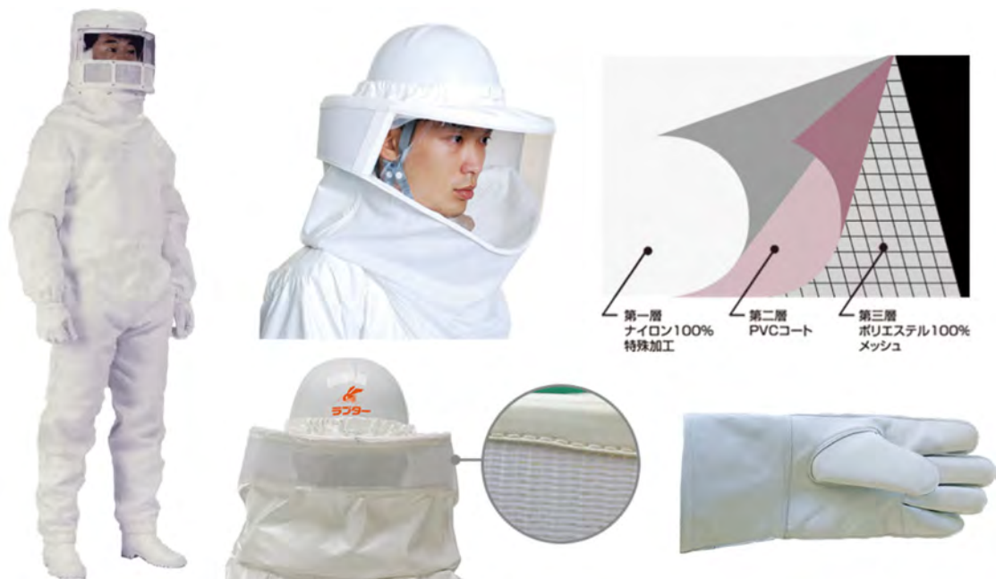
Figure 4-5. Protective gear designed to protect the wearer from hornet stings. The suit is made from a material that is slick on the outside to prevent hornets from being able to hold on to the suit. This material is made of multiple layers and thick enough to prevent the sting from penetrating. Unlike a beekeeper's mesh veil, the visor on a hornet suit is made of hard plastic and the back is a thick, reinforced material. Photo credits: asuka21.blue.coocan.jp and www.dic-corp.co.jp/contents/raptor.html.
